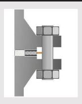
The FRG enables bolted joints to be easily and effectively sealed to prevent internal corrosion. The soft SIGMA inner ring of the FRGs conform seamlessly to the flange face, even if already damaged to:
